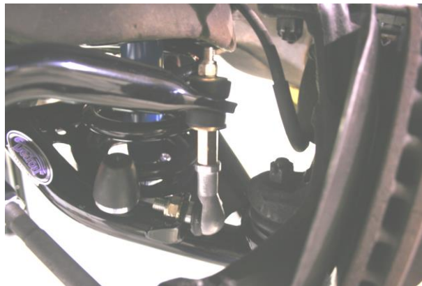
Figure 2 - End Link Installed
