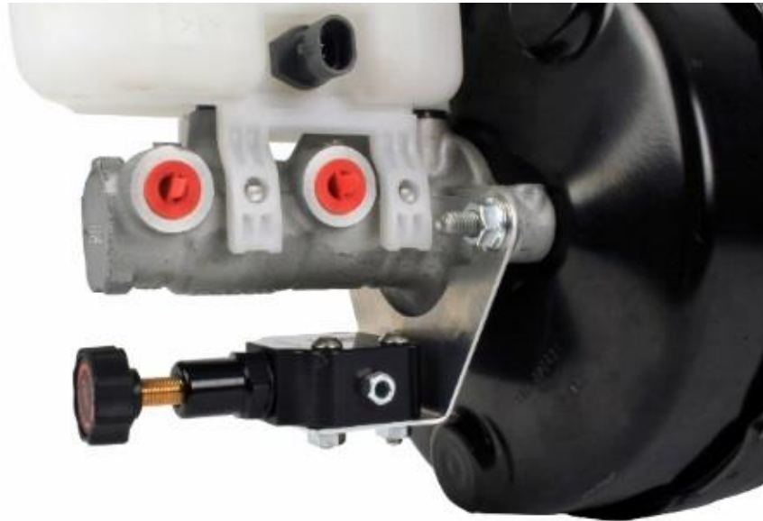
Figure 1 - Completed Bracket Installation
