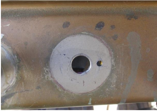
Figure 5 - Drill Anti-Rotation Hole
