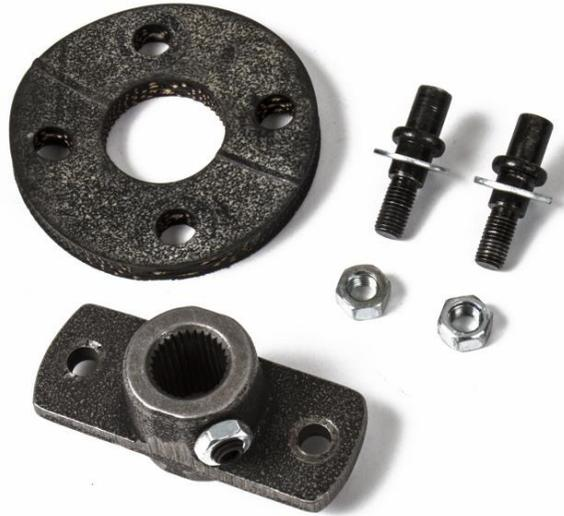
Figure 2 - Separate the Rag Joint from the Coupler
